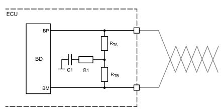
NOTE: The serial RC combination (R1, C1) at the center tap of the split termination provides a termination to GND for common mode signals. R1 is preferably omitted. Typical values are given in the following table.
