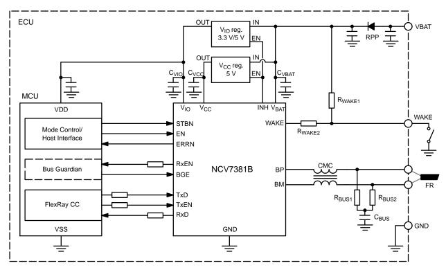
Figure 17. Typical Application Diagram
