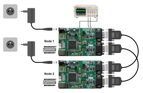
Figure 2. Getting started setup connection
