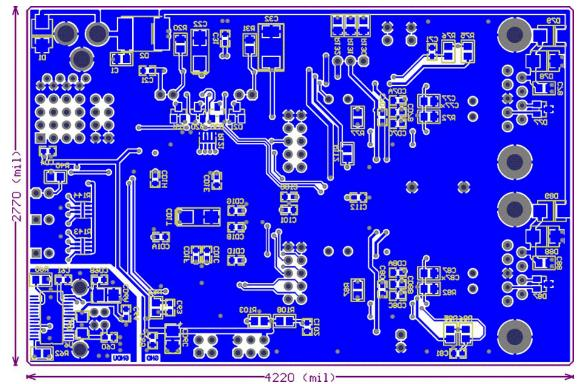
Figure 29. PCB Bottom Composite Drawing (Mirrored)
