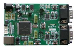
Figure 1. NCV7381B0V2GEVB Evaluation Board
