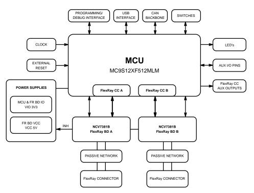
Figure 16. NCV7381B EVB Block Diagram
