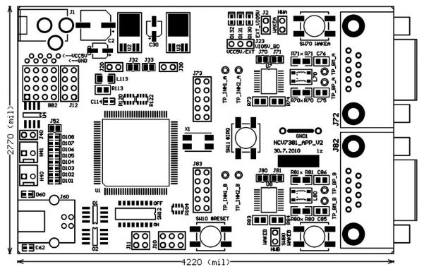
Figure 26. PCB Top Assembly Drawing
