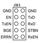
Figure 11. FlexRay BD Digital Signals Test Points Headers
