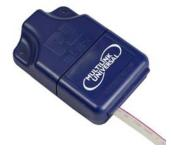
Figure 23. PEmicro USB Multilink Universal Debug module
