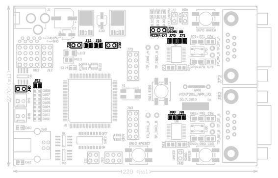
Figure 12. Jumpers and Soldering Straps
