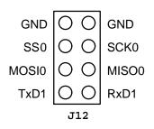
Figure 7. Aux Digital I/O Connector
