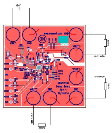
Figure 5. NCV97311A Board Connections
