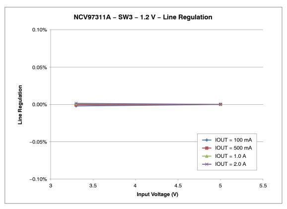
Figure 11. Line Regulation for SW3 with a 1.2 V Output
