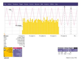
The modulation depth and modulation frequency are each set by 2 external resistors to GND. The modulation frequency can be set from 5 kHz up to 50 kHz using a resistor from the RMOD pin to GND. The modulation depth can be set from 3% up to 30% of the nominal switching frequency using a resistor from the RDEPTH pin to GND. Please see the curves below for typical values:
