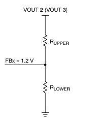
The upper resistor is set to  $10 \text{ k}\Omega$  and is part of the feedback loop. To maintain stability over all conditions, it is recommended to change the only the lower feedback resistor to set the output voltage. Use the following equation:
