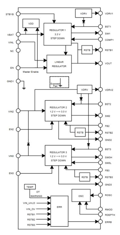
Figure 2. NCV97311A Block Diagram
