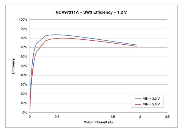
Figure 8. Efficiency for SW3 with a 1.2 V Output
