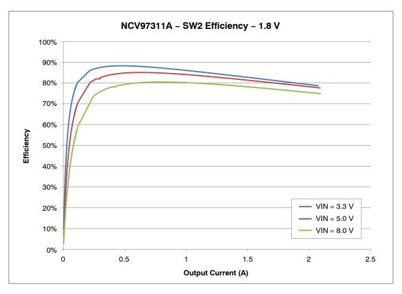
Figure 7. Efficiency for SW2 with a 1.8 V Output
