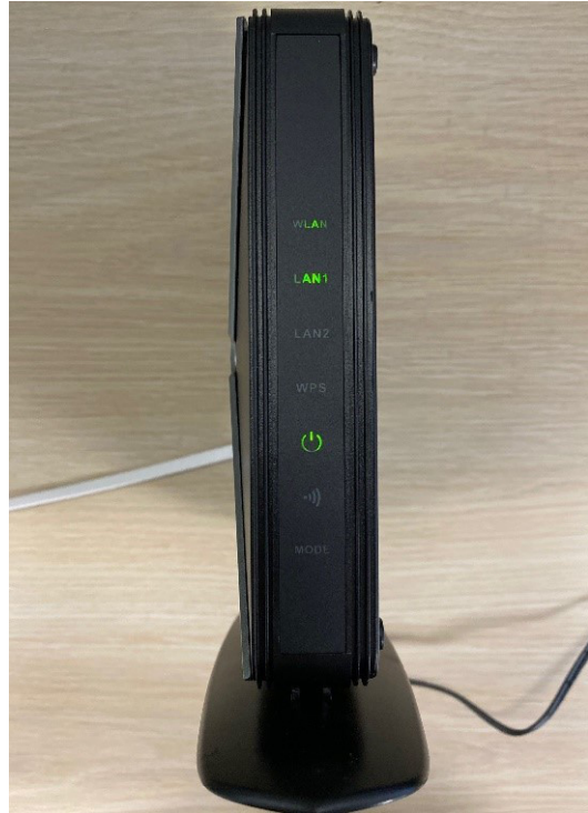
Figure 3. Console Display When QBOX840-5S7-GEVK Successfully Boots Up
