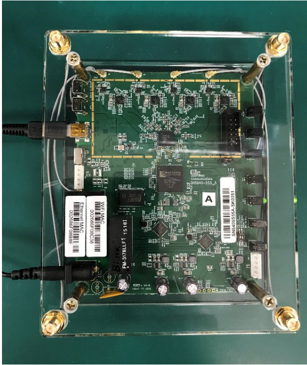
Figure 5. LED Indication When QHS840-5S5-GEVK Powers Up
