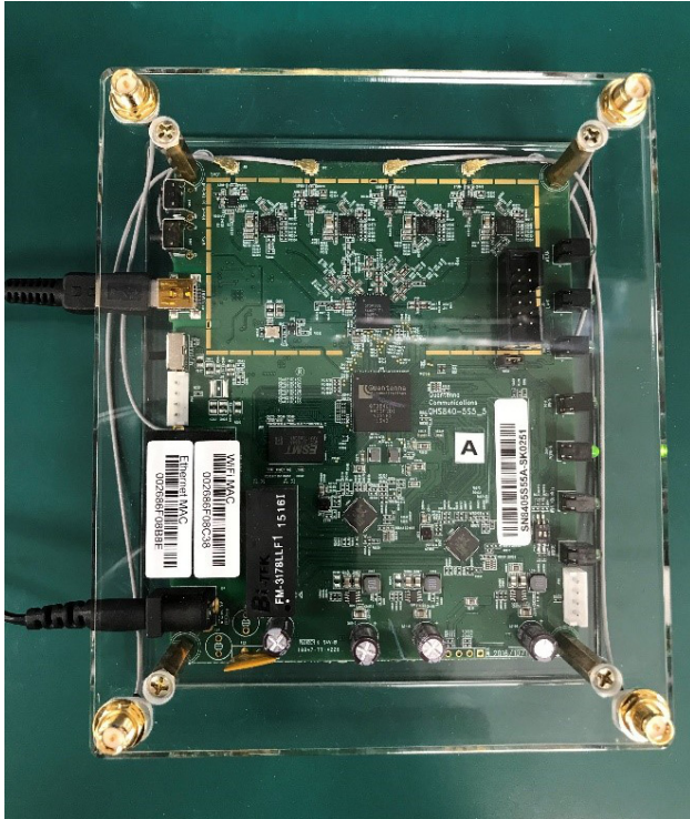
Figure 5. LED Indication When QHS840-5S5-GEVK Powers Up
