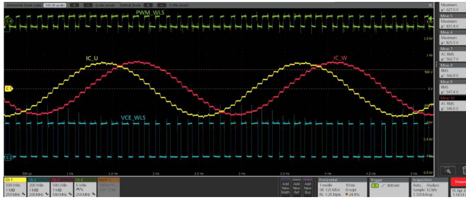
Figure 13. Switching Waveforms, C1: U Phase Current; C2: W Phase Voltage (Low Side Switch); C3: W Phase Current; C4: Input PWM Signal (W Phase Low Side)
