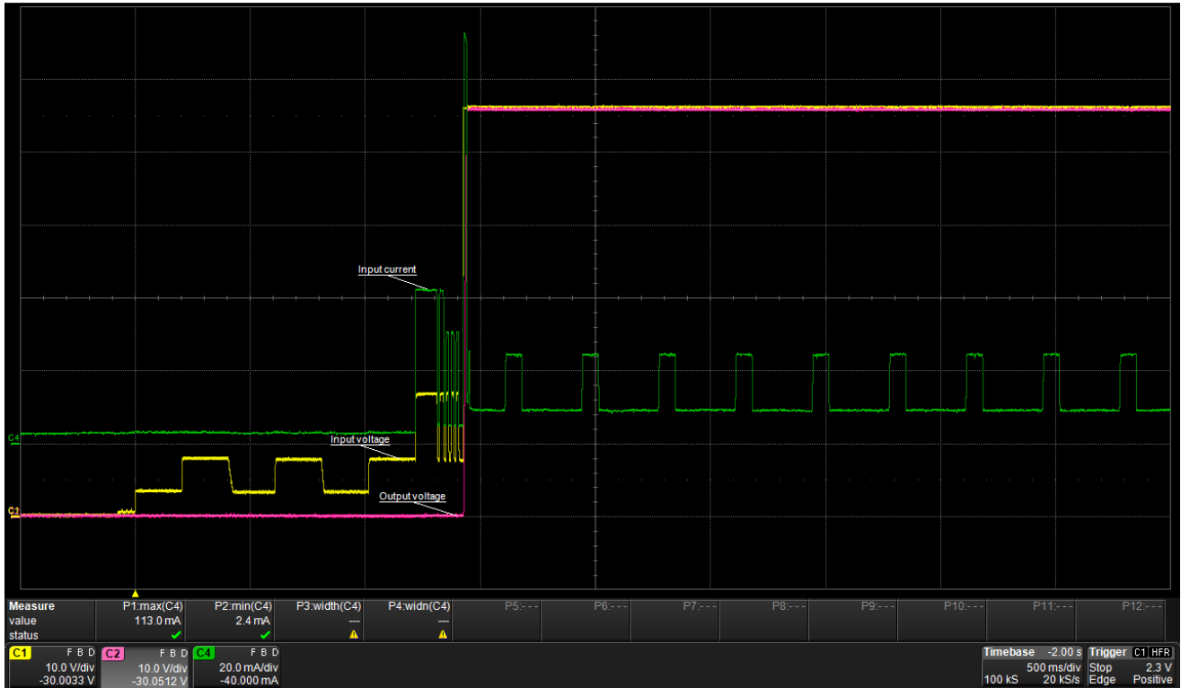
Figure 17. No Load Start-up, MPS Circuit Turned ON
