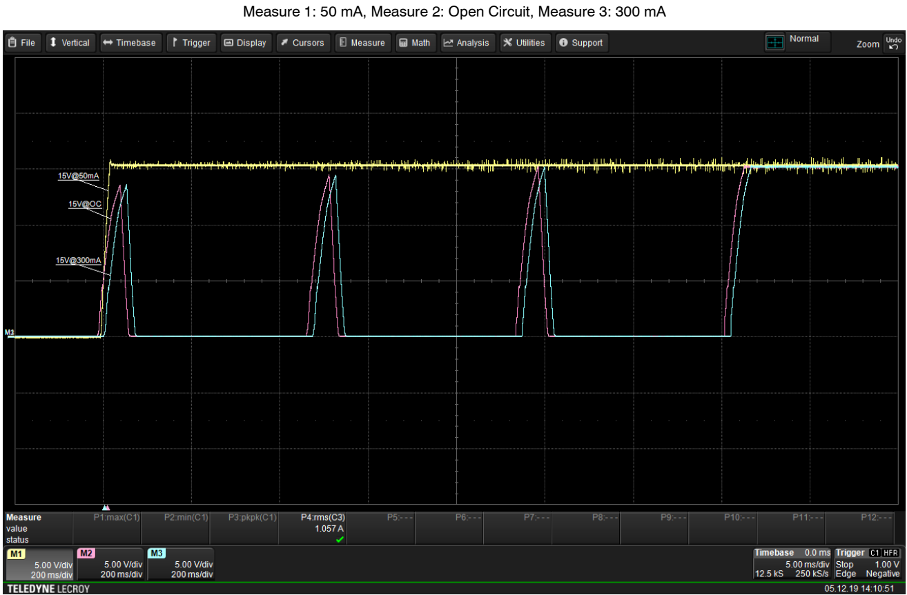
Figure 28. Start Up to Open Circuit, to 50 mA and to 300 mA at 390 V DC Input
