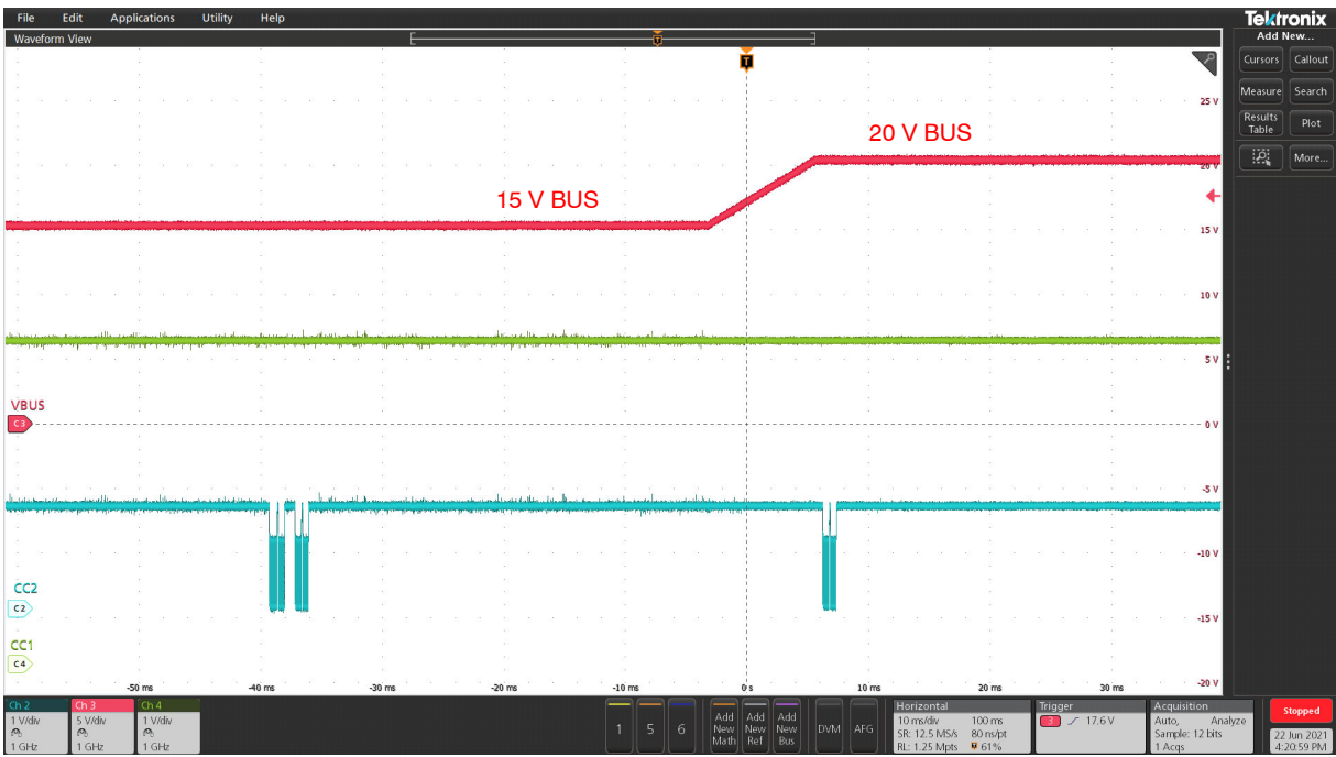
Figure 8. Sink Request 20 V PDO, CC = CC2, VCONN = CC1
