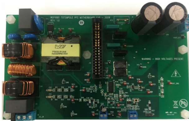
Figure 1. NCP1680 Evaluation Board
