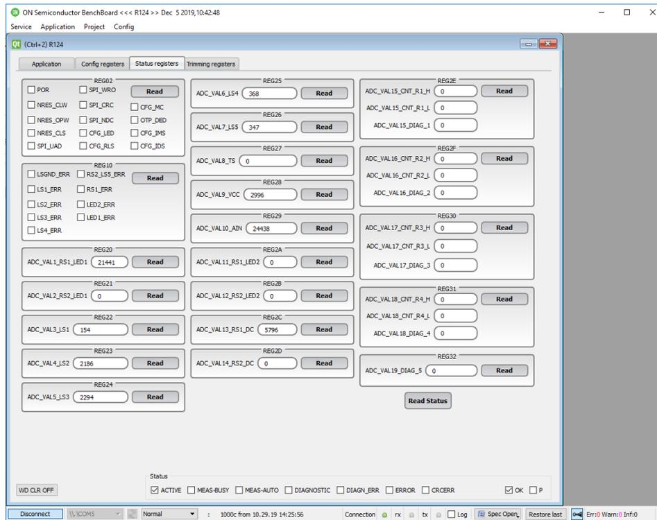
Special attention can be taken to the Reg02 register. Configuration errors are shown here. Most of the times, when the measurement will not start, this status register will
