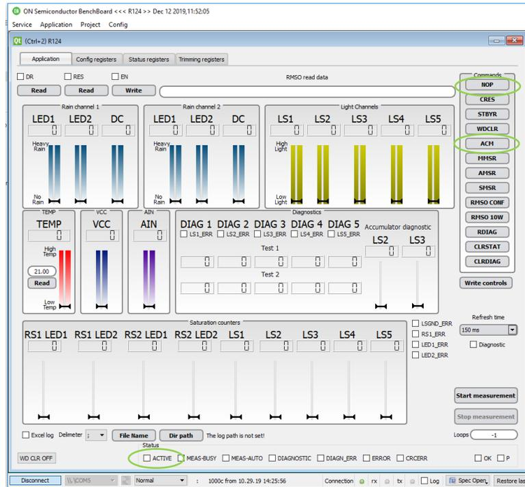
– A “MMSR”, manual measurement can be started now. Clicking the “RMSO CONF” button to read the configured measurement registers from the chip. The values are presented in the Status register screen (next page shown).
