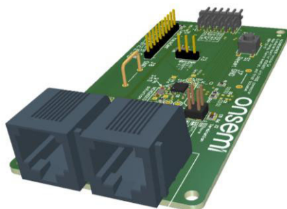
Figure 7. SPE Connector on Revision-2 Boards: Alternative 1, RJ45
