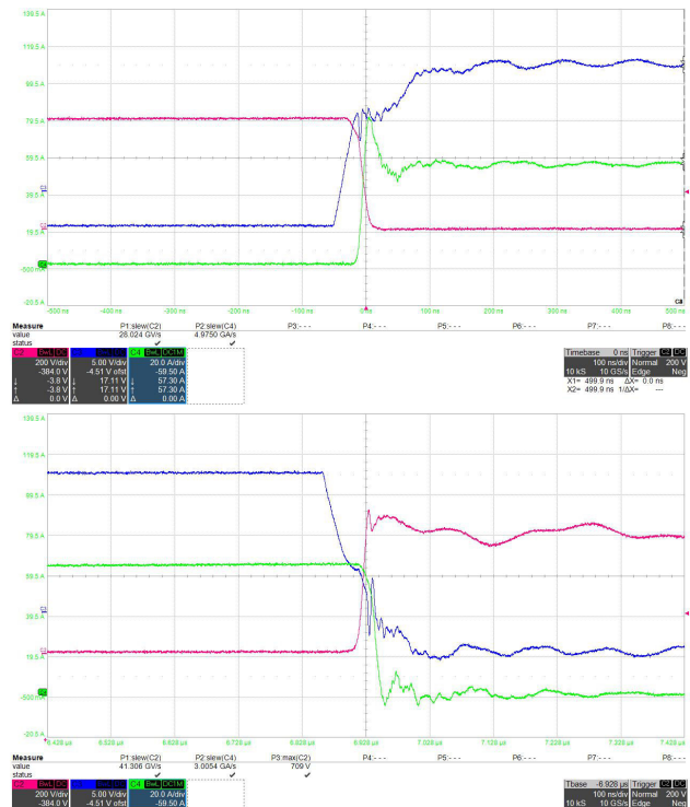
Figure 8. Switching Waveforms – Green Id, Red Vds, Blue Vgs
