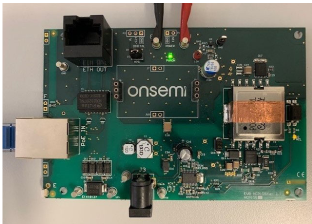
Figure 1. Operational NCP1081REF12VC4GEVB showing Basic Interconnections
