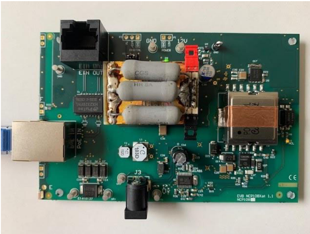
Figure 13. Emission Test DUT: NCP1081REF12VGEVB with 7.3 \Omega Load
