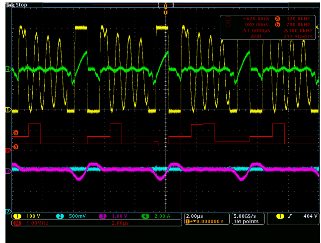
LLC Waveform at Light-load Mode 2 A Load – Package detail
