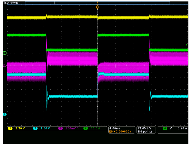
LLC Waveform – Step response 2 A → 15 A
