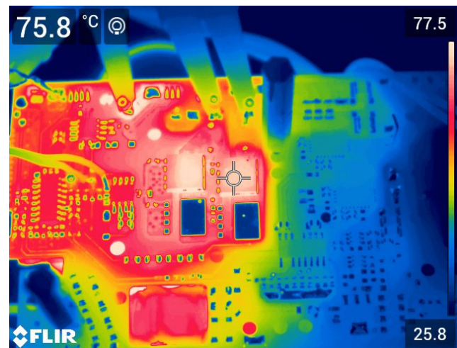
TP-PFC Inductor magnetic core Thermal Image
