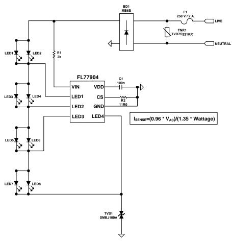
Figure 2. Typical Application Circuit of the 8 W Evaluation Board
