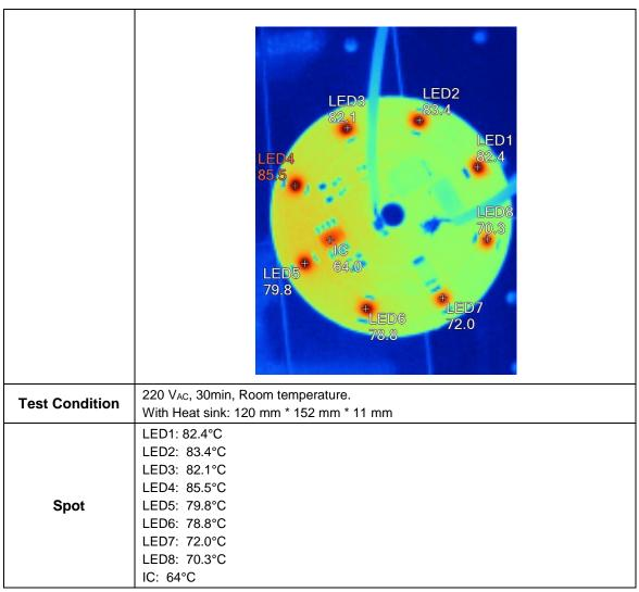
Temperatures on all components at high line evaluation board are less than 85°C. The IC's temperature is lower than 75°C. Measured temperature can be changed with dimension of heat sink.
