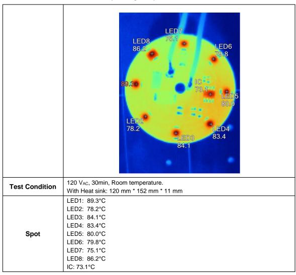
Temperatures on all components at low line evaluation board are less than 90°C. The IC's temperature is lower than 75°C. Measured temperature can be changed by dimension of heat sink.
