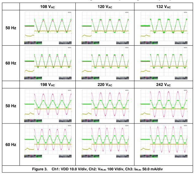
Table 8 shows overall startup performance at each line input voltage with 50 / 60 Hz. Input current flows immediately when input voltage is applied.
