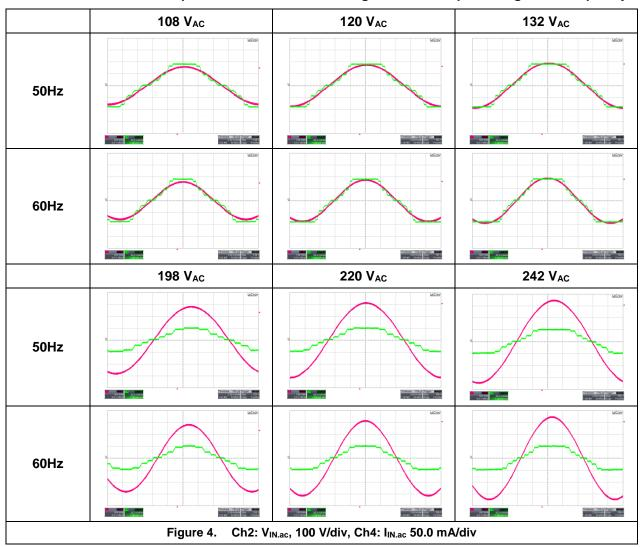
Table 9 shows overall normal operation performance at each line input voltage with 50 / 60 Hz. When input voltage is higher than all string LED forward voltage, LED 4 pin can be conducted and its time depends on input voltage and line frequency.
