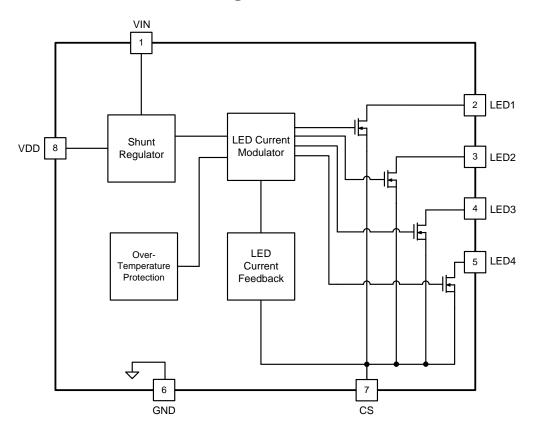
Figure 1. Simplified FL77904 Block Diagram
