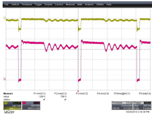
Figure 18. V_{DS}=786\text{ V} , V_{DIODE}=249\text{ V} , Steady-State, Full-Load Condition, 460\text{ V}_{AC} , (CH1: V_{DIODE} (200 V/div), CH2: V_{DS} (200 V/div), Time: 5 μs/div)
