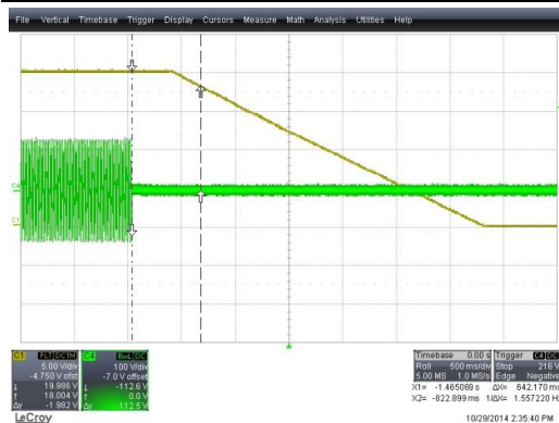
Figure 33. t_{HOLD} = 0.6 \text{ s} , 85 V AC , (CH1: V_{OUT} (5 V/div), CH4: V AC (100 V/div), Time: 500 ms/div)
