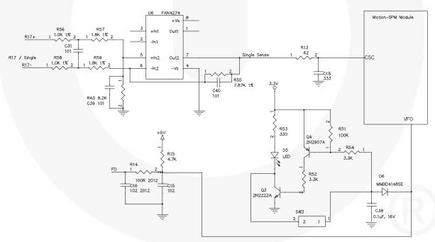
Figure 20. Short-Circuit Protection Circuit
