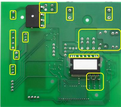
Figure 5. High-Voltage Areas (Bottom Side)
