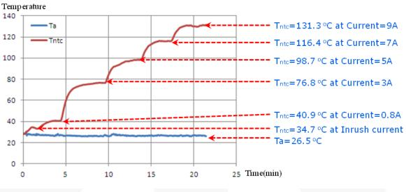
RT1 operating temperature measured at varying load currents.
