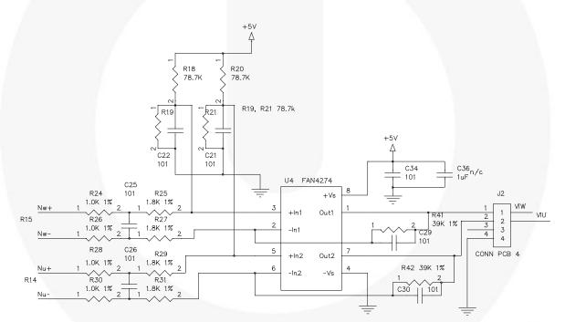
Figure 19. Current-Sensing Circuit
