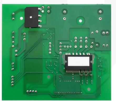
Figure 2. Bottom View, 140 mm x 160 mm
