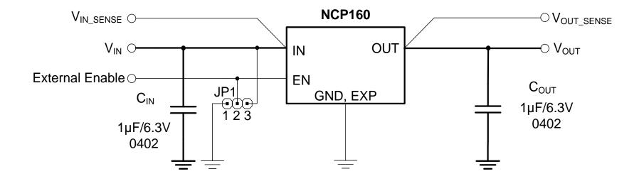
The NCP160 is 250mA high performance LDO with low quiescent current (23µA max.) and very high PSRR. The NCP160 also offers excellent load/line transients and ultra-low noise.
