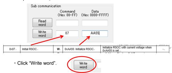
Note: The accuracy of the Initialization requires the OCV reading to be taken with minimal load or charge, under 0.025C, on the battery. (i.e. less than 75mA for 3000mAh design capacity battery.)
