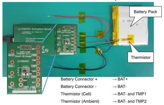
Note:  $10 \text{ k}\Omega$  NTC thermistor is required.
