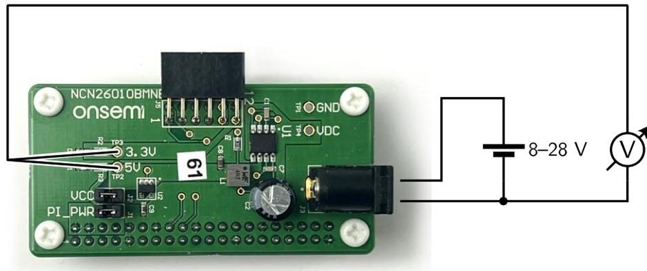
Figure 1: Test setup for revision-1 boards (shown without test board).
