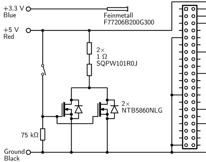
Figure 3: Schematic of the test board.
