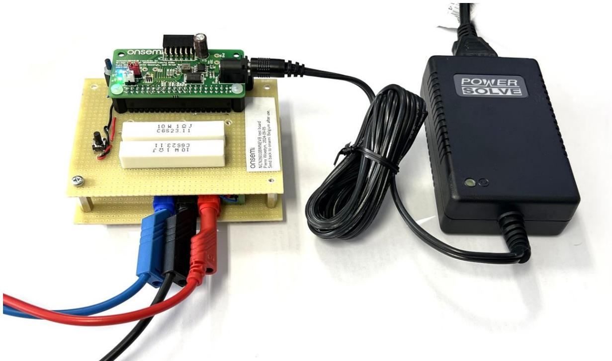
Figure 2: Test setup for revision-2 boards (shown with test board).
