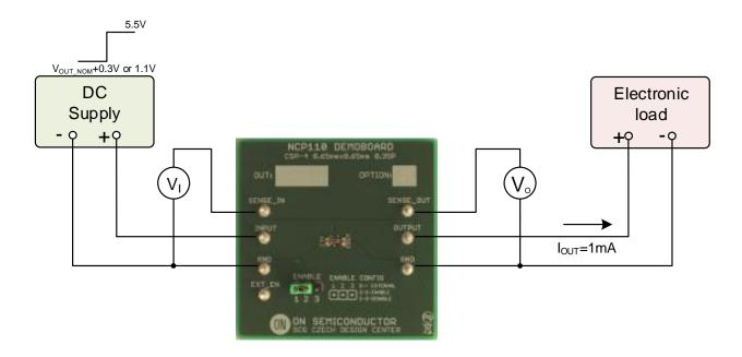
Figure 3: Test configuration for measurement REG<sub>LINE</sub>, Line Regulation
