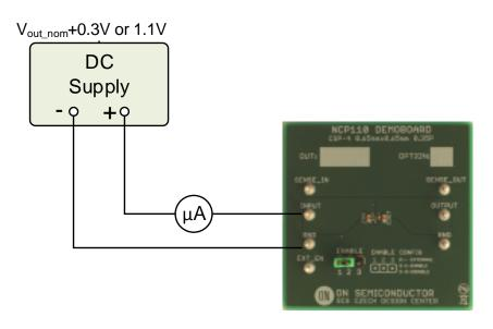
Figure 1: Test configuration for measurement IQ, Quiescent Current
