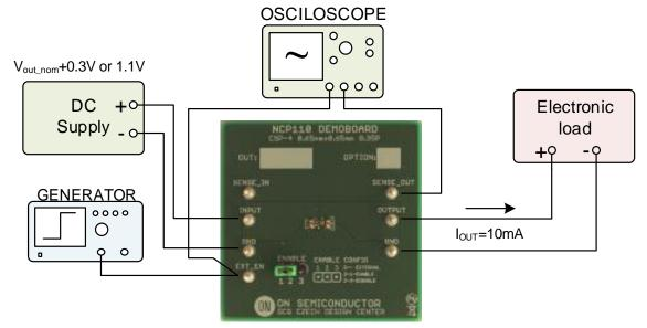
Figure 4: Test configuration for measurement enables response
