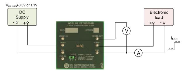
Figure 2: Test configuration for measurement REG<sub>LOAD</sub>, Load Regulation
