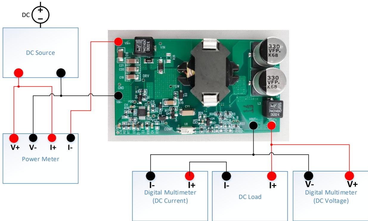
Figure 1 - Test Configuration
