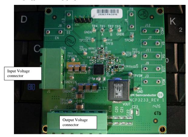
For operation at input voltages greater than 5 V, reverse the prior settings, i.e., open J2 and J3 and short J1, and install the zero- $\Omega$  resistor into R14. The EVB should now be configured to operate from 5 V to the maximum input voltage for the EVB (~21 V).
