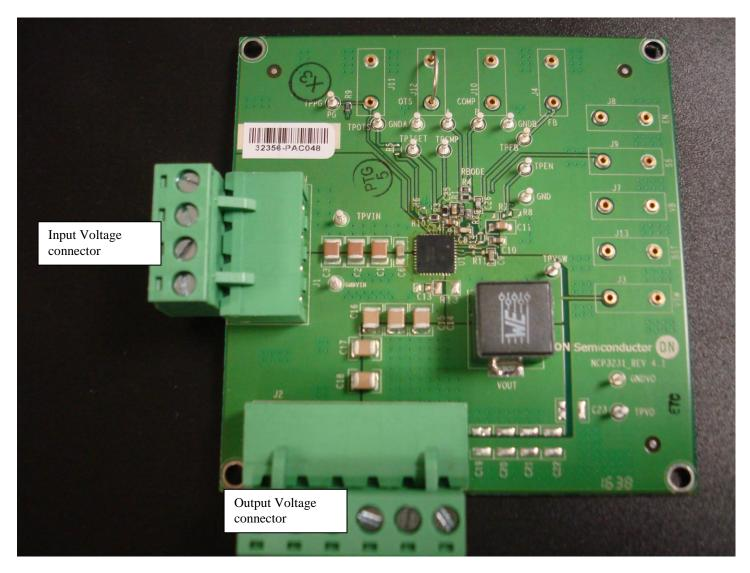
The EVB has two large green receptacles – one 4-pin (J1) for input voltage and one 6-pin (J2) for output voltage. The mating connectors should have been shipped with the board. The mating connectors have screw terminal connections to allow single wires to be attached to the connector pins and then the connector can be plugged into the corresponding receptacle on the
