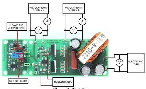
Figure 1: Test Setup
