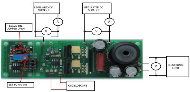
Figure 1: Test Setup
