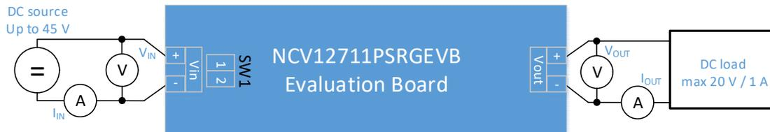
Figure 1: Test Setup
