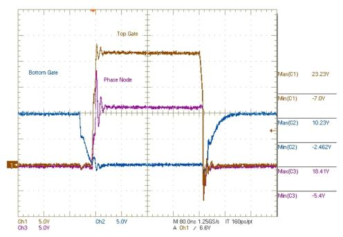
Figure 9: Switch Node Waveforms for Vdrvr = 10V
