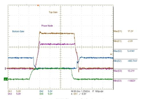
Figure 10: PWM Signal at G1 for Iout = 0A
