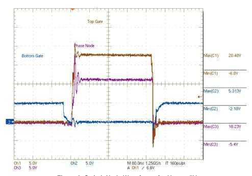
Figure 8: Switch Node Waveforms for Vdrvr = 5V
