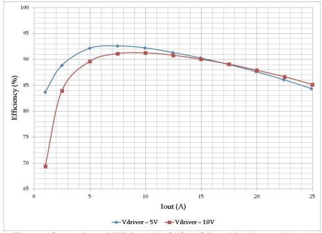
Figure 5: Comparison of Efficiency for ONS321G Board for Vdrvr = 5V & 10V
