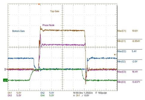
Figure 11: PWM signal at G1 for Iout = 20A
