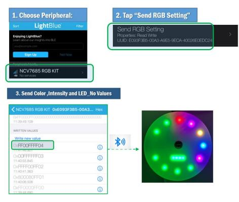
Figure 6. Using 'Light Blue' App to control the board
