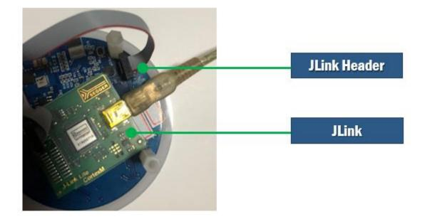
4. Launch "Flash Loader" and load "RGB\_1V6F.hex" file to finish programming.
