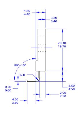
A. THIS PACKAGE DOES NOT CONFORM TO ANY STANDARDS. B. ALL DIMENSIONS ARE IN MILLIMETERS. C. DIMENSIONS ARE EXCLUSIVE OF BURRS, MOLD FLASH AND TIE BAR PROTRUSIONS.
