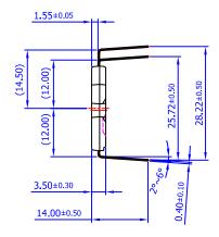
NOTES: UNLESS OTHERWISE SPECIFIED A) THIS PACKAGE DOES NOT COMPLY TO ANY CURRENT PACKAGING STANDARD B) ALL DIMENSIONS ARE IN MILLIMETERS C) DIMENSIONS ARE EXCLUSIVE OF BURRS, MOLD FLASH, AND TIE BAR EXTRUSIONS D) ( ) IS REFERENCE
