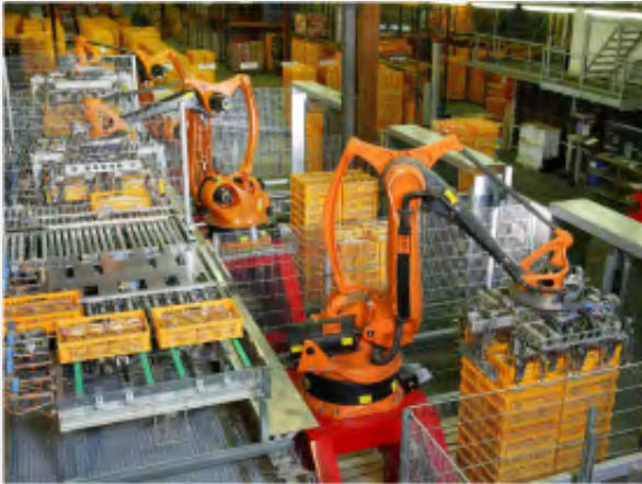
An articulated robot produced by KUKA Roboter GmbH for a bakery in Germany. [Public domain image]
