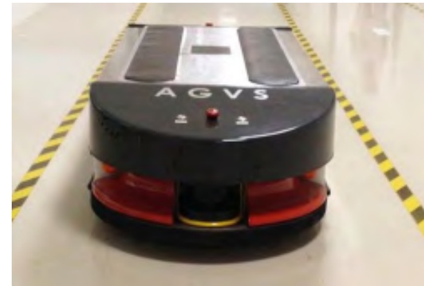
A hospital transporter that stays inside its boundary strips. [Hospital La Fe de Valencia, photo by Mgonezrobotnik, CC 4.0]
