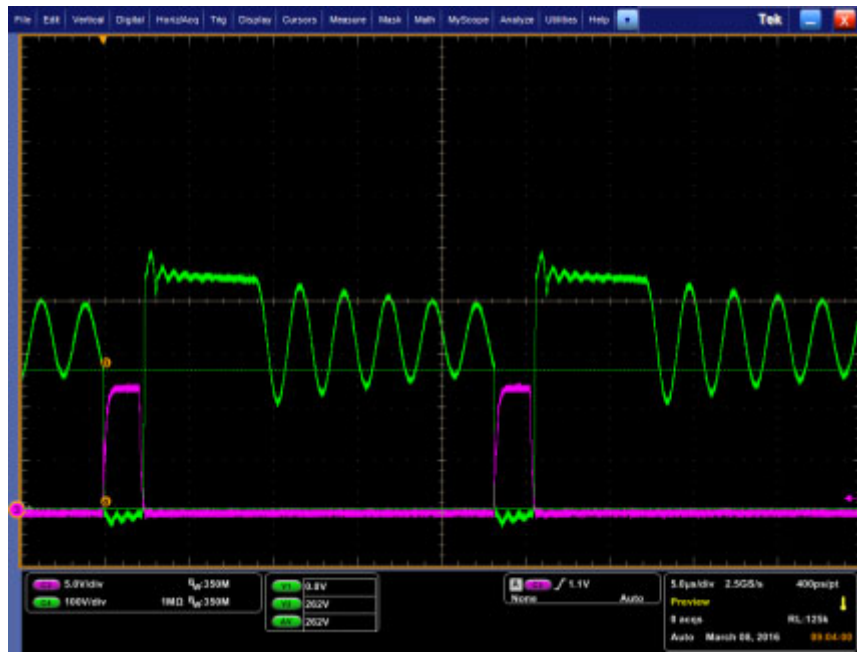
Figure 7. Valley Switching at 6 th Valley for Improved Efficiency (Green: Drain voltage, Purple: Drive)
