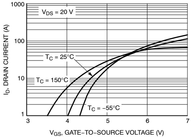
Figure 2. Transfer Characteristics
