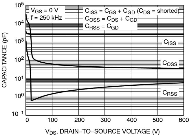
Figure 5. Capacitance Characteristics
