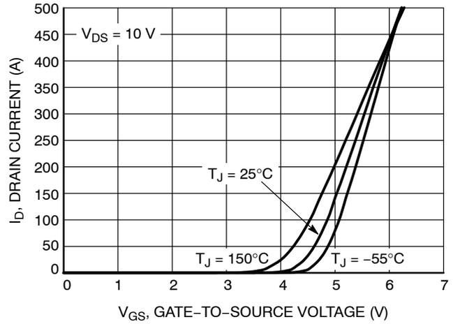
Figure 2. Transfer Characteristics
