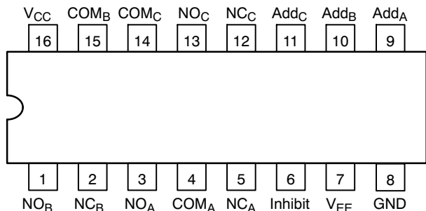
Figure 1. Pin Connection (Top View)
