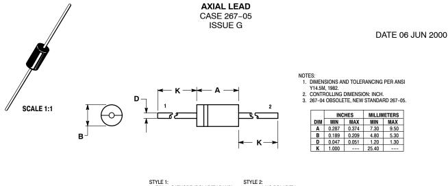
STYLE 1: STYLE 2 PIN 1. CATHODE (POLARITY BAND) 2. ANODE
