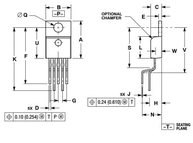
NOTES: 1. DIMENSIONING AND TOLERANCING PER ANSI Y14.5M, 1982. 2. CONTROLLING DIMENSION: INCH.
