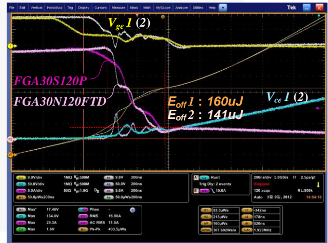
Figure 8. Switching Performance Comparison
