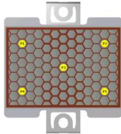
Figure 5. PCM Measurement Point: F2 Modules
