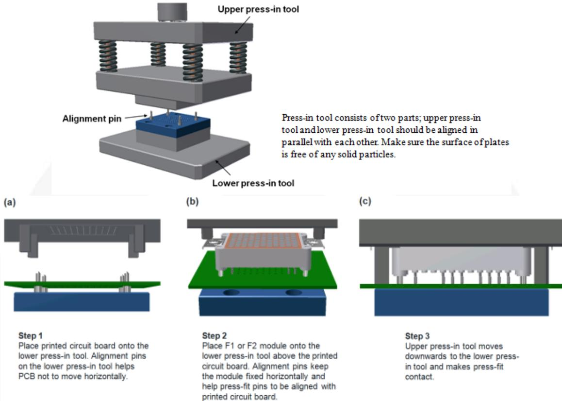
**Figure 9. Sequence of Press-in Process (with PCM Spacer)**
