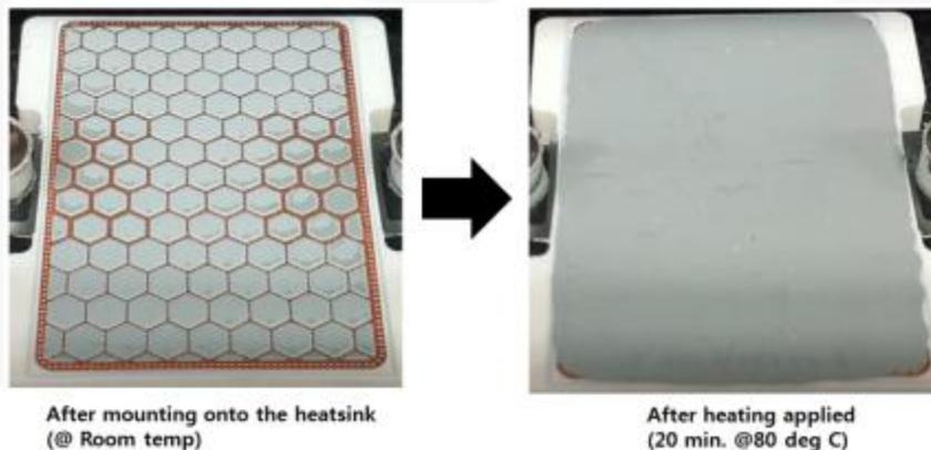
Figure 6. Appearance of PCM Distribution through Glass Inspection Block Under Phase Change Temperature
