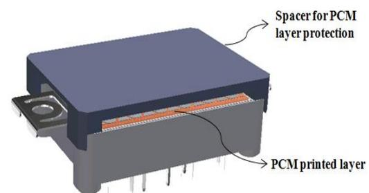
Figure 8. Example of Spacer to Protect PCM Printed Layer during Soldering Process
