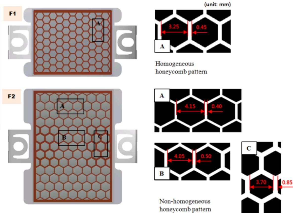
**Figure 3. PCM Stencil Geometry Applied on F1 and F2 Modules**
