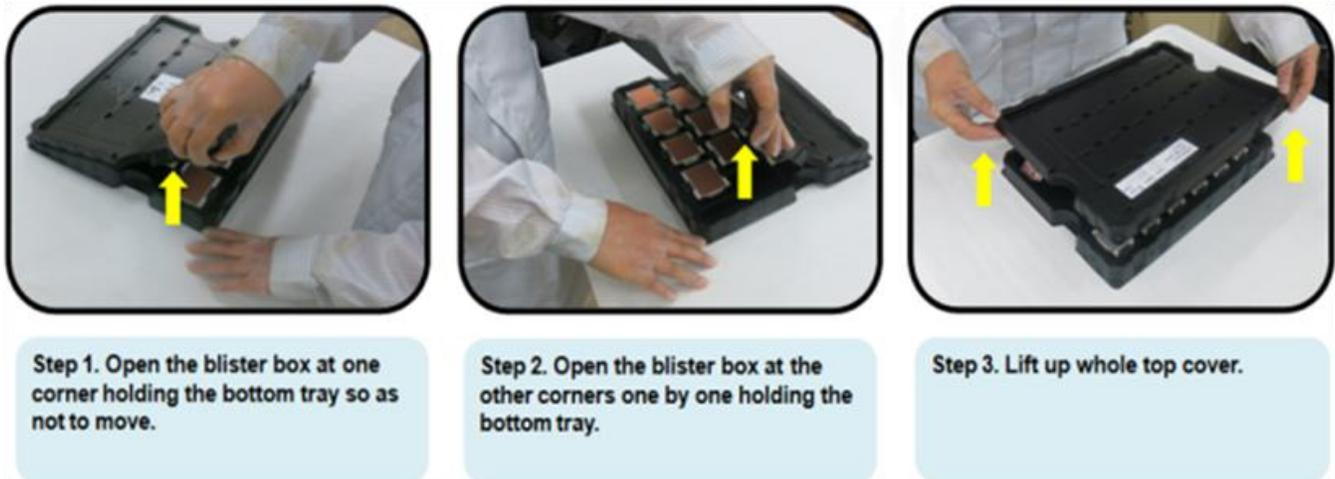
**Figure 12. Recommended Opening Procedure of Tray Box**
