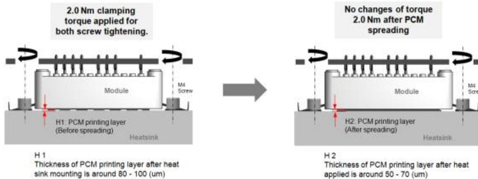
Figure 7. PCM Settling Process
