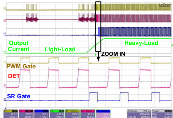
Figure 10. Test Waveforms for Load Change (Light Load to Heavy Load)
