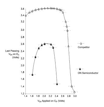
Figure 10. Inverting Function Data/Clock V<sub>IH</sub> Noise Margin Competitor vs. ON Semiconductor 5.0 V V<sub>DD</sub> at  $25^{\circ}$ C
