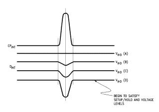
Figure 7. Data Input Level Can Cause Output Errors
