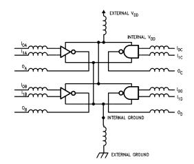
Figure 1. A Typical 2–Input Quad NAND Gate
