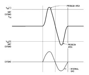
Figure 3. Ground Bounce Changes Input Threshold
