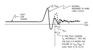
Figure 8. Ground Bounce Causes Dynamic Threshold
