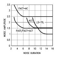
Figure 4. Device Speed Effects Noise Margins
