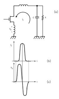
Figure 2. Package Inductance Causes Ground Bounce
