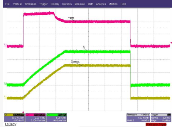
Figure 14. Current Limit Waveforms
