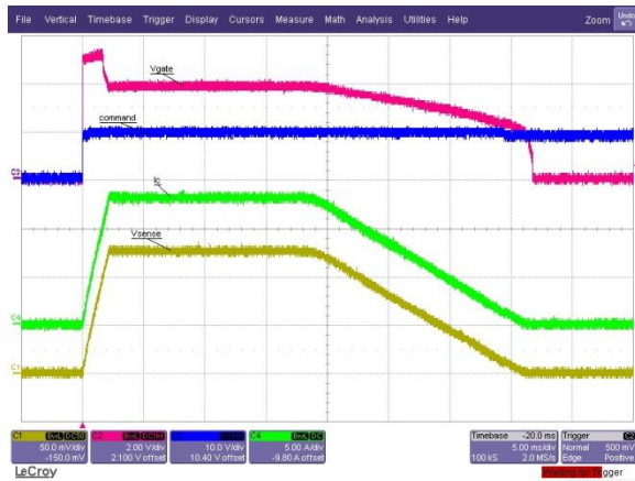
Figure 15. Soft Shutdown (SSD) Waveforms
