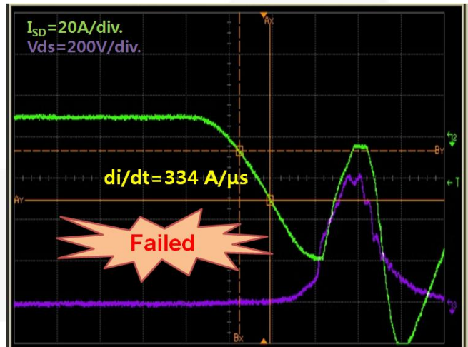
(b) Competitor A MOSFET Failing Waveforms During Body Diode Reverse Recovery
