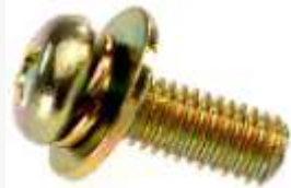
Figure 13. SEMS Screw (Size M3, Spring Washer 5.0Φ, Plain Washer 7.5Φ)
