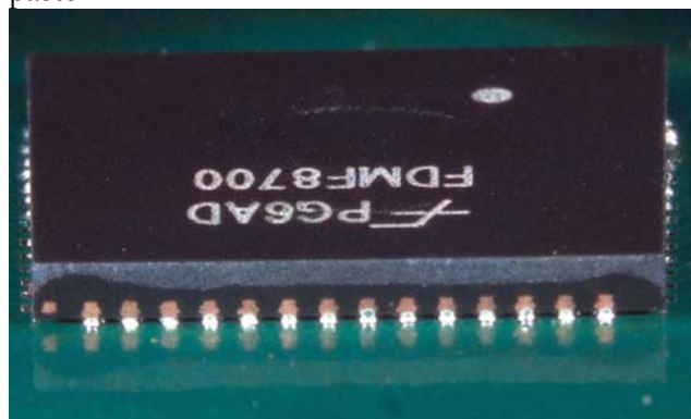
Figure 2: Exposed copper on package edge from singulation process.
