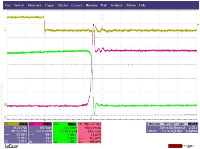
Figure 3. IGBT Turn-Off Switching Waveform Comparison [Ver. 2.0 IGBT Turn Off]
