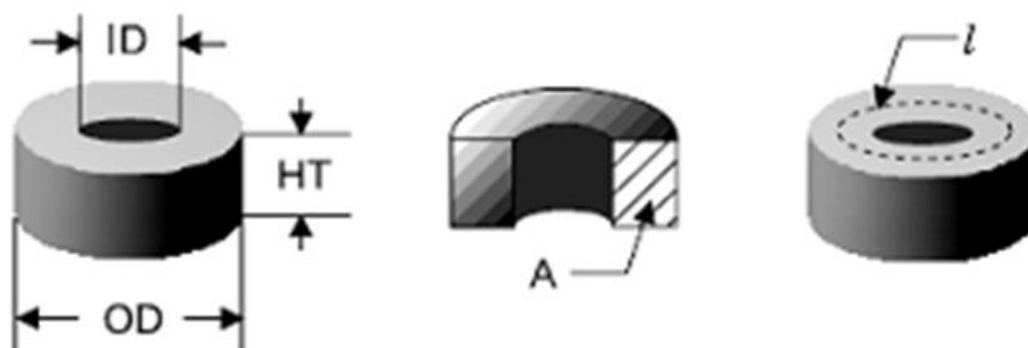
Figure 2. Specification of the Selected Toroidal Core: CK740060C
