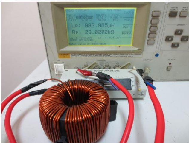
Figure 7. Inductance of Inductor (0.98 mH)
