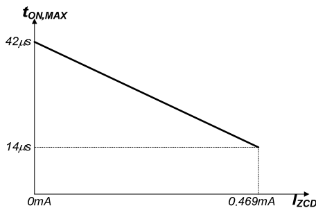
Figure 21. Maximum On-Time Variation vs. I_{ZCD}
