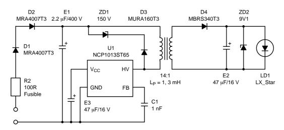
Figure 2. Complete Schematic Diagram of the LED Flasher
